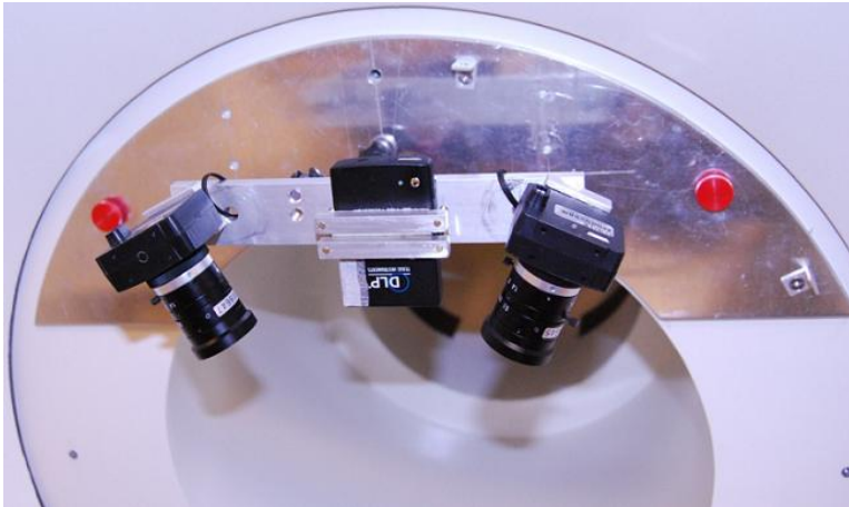
Figure 4.1: The structured light scanner mounted on the HRRT
