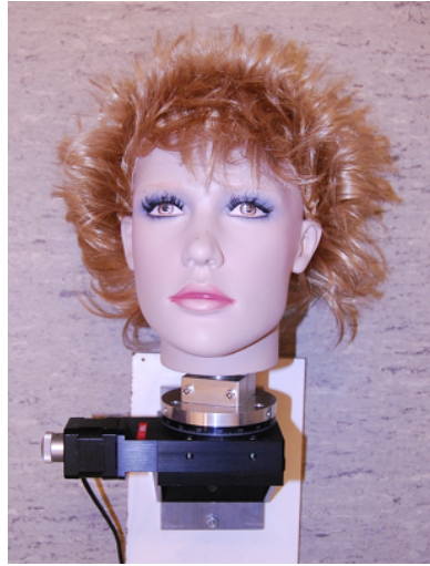
Figure 4.3: The mannequin head and the motor.
