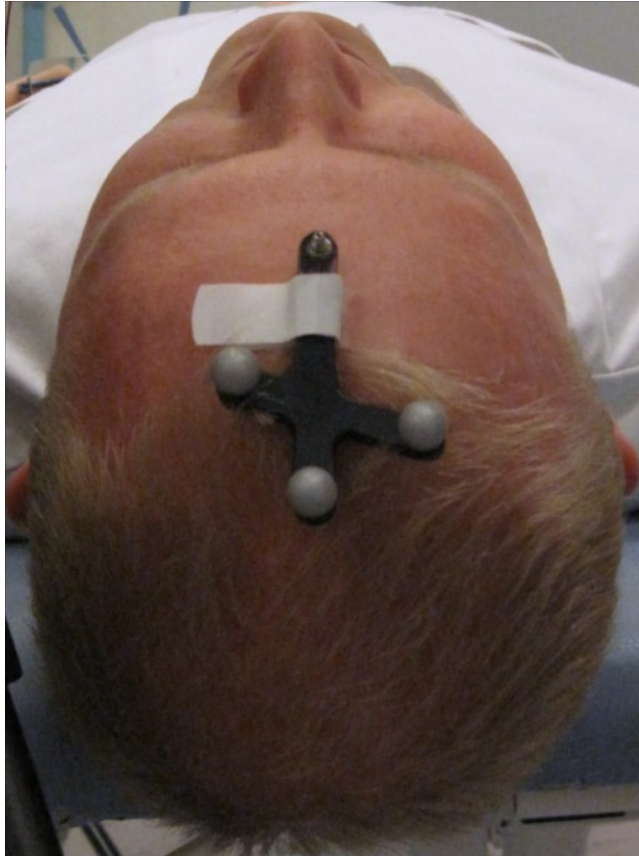
Figure 6.2: The head of the human subject for experiment II with the Polaris rigid body tool attached using a Velcro band-aid – see Olesen 2009 [28].
